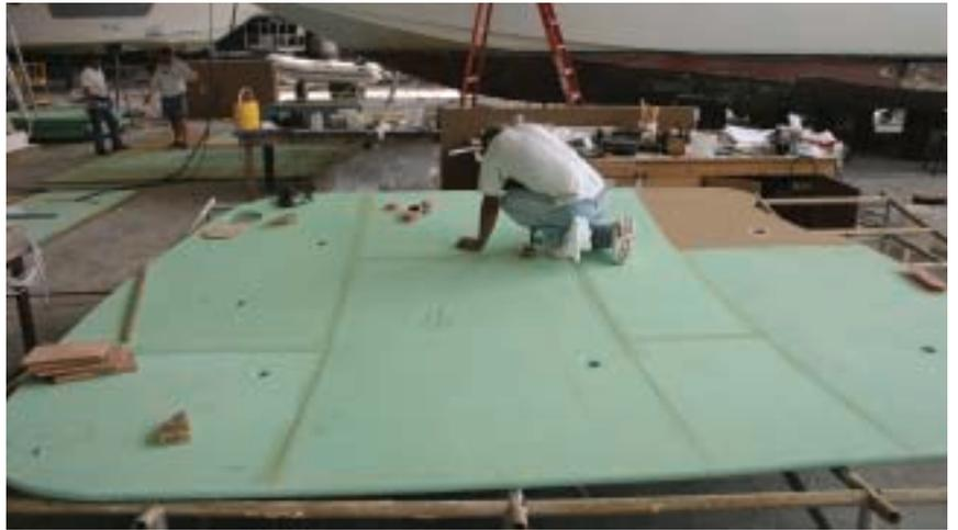
A lightweight hard top is being fabricated for a 40-foot Cabo.
