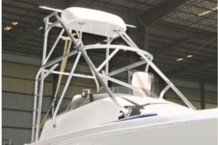
A 31 Contender Fisharound is being outfitted with a low profile tower and hard top, along with riggers and tower controls
