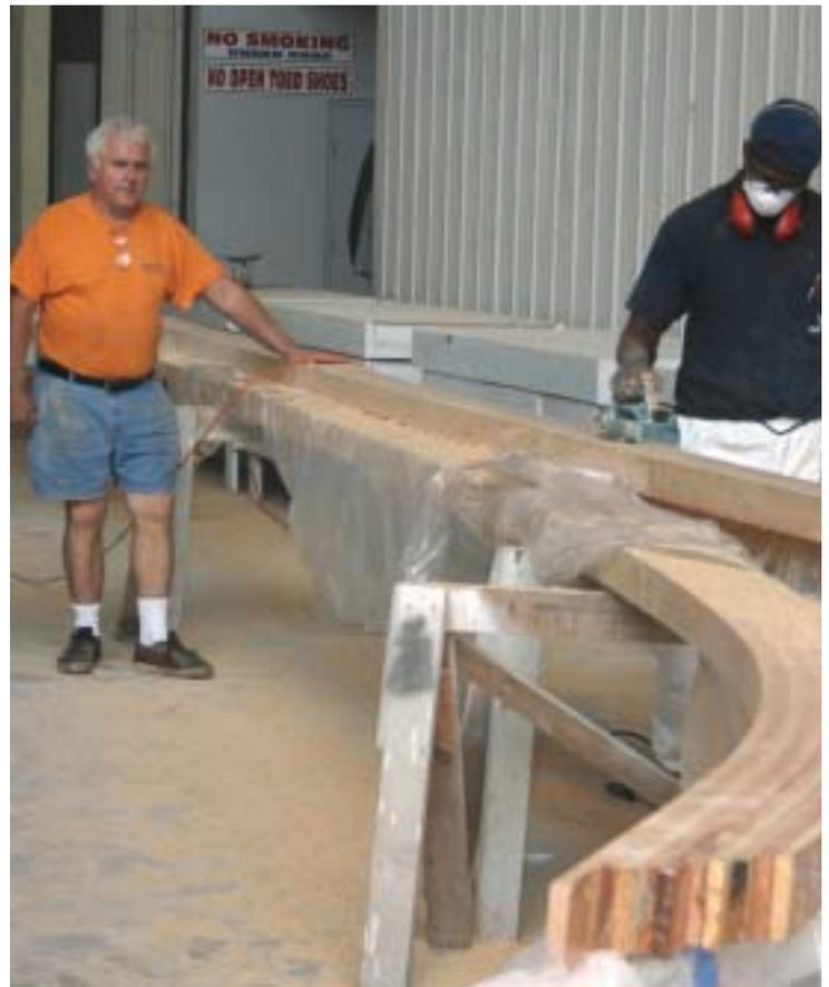
*Hull Construction Foreman John Carver oversees the early stages of construction of the new 68-foot FREEDOM, monitoring the fabrication of the keel and stringers.*
