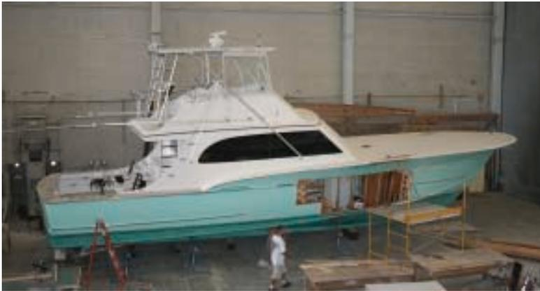
No thanks to Hurricane Wilma, ACY is repairing damage to the hull and forward engine room, and installing new carpeting on the BABY GRAND, a 61' Ricky Scarborough.
