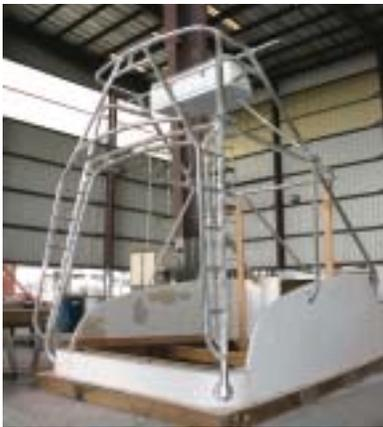
This low profile tower is being fabricated on a jig for a new 33' L&H walkaround.
