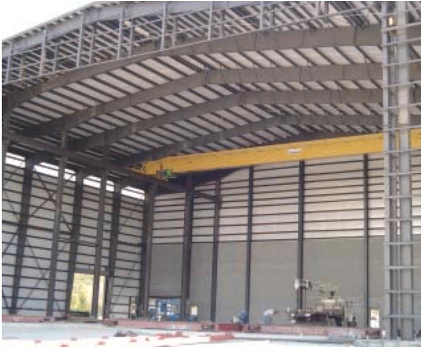
The remote-controlled crane to be used in tower fabrication is visibly mounted on the yellow guide beam along the ceiling.
