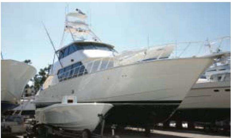
LIGHTWAVE, an 86' Hatteras sportfisherman, has returned to ACY to upgrade its water lines to Unipipe®, flush the fuel tanks, repair the air compressor system and replace the deck hatches. Additional routine service includes teak deck refinishing, a hull wax and a full bottom job.
