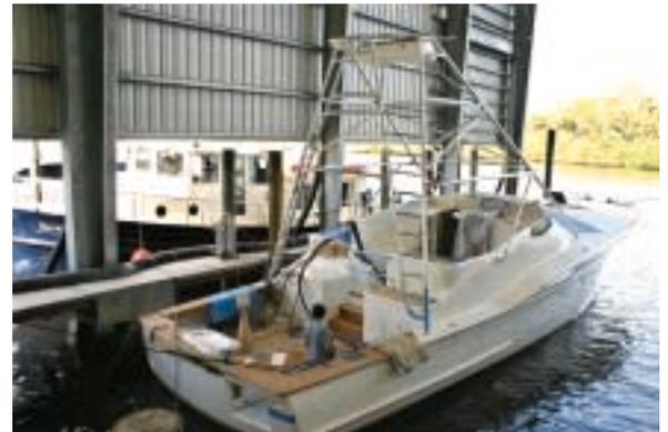
Having completed the interior fabrication, engine installation and a complete paint job, ACY is now putting the finishing touches on this new custom-built 50' express sportfisherman with the installation of a BAT tower and electronics package by IMS. The project has been directed every step of the way by the boat's owner, Neil Afromsky, who brought the unique vessel shell – designed by Applied Concepts – to ACY for finishing.
