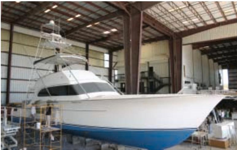
ACY is closing the davit hole on the foredeck, refinishing the bow hatches and fabricating new custom vent boxes on HEADS UP, a 61' Buddy Davis.
