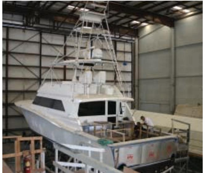
SALT SHAKER, a 65' Jim Smith, is undergoing a major overhaul at ACY. Work includes engine room and lazzarette fuel tank replacement, a new fuel plumbing system, running gear replacement, tower repair, as well as major mechanical and electrical system upgrades.
